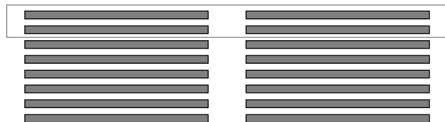
Figure 4-2 Memory slots on an MK401; the dotted region shows one of the 4 groups of 4 memory slots.
